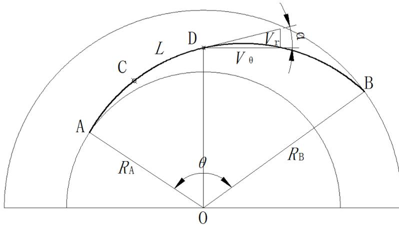
Figure 9 Streamline in the vaneless diffuser
