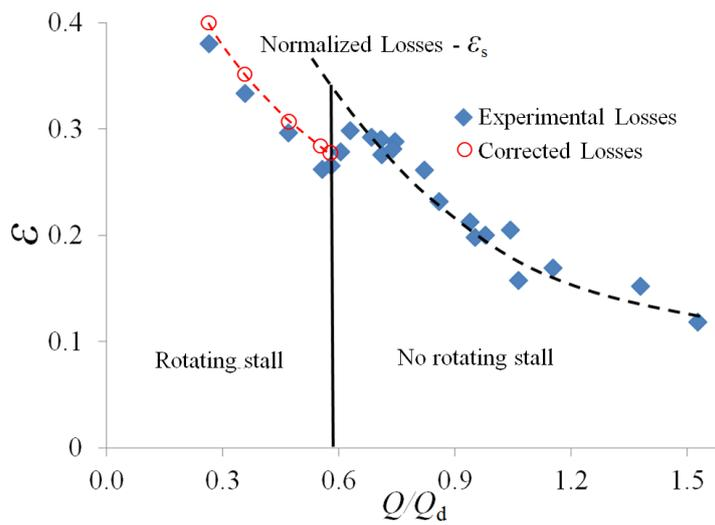
Figure 18 Comparison between experimental losses and corrected losses
