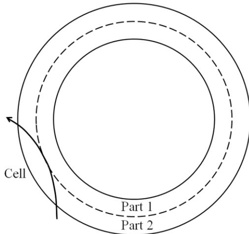
Figure 16 Two assumed spaces in the vaneless diffuser
