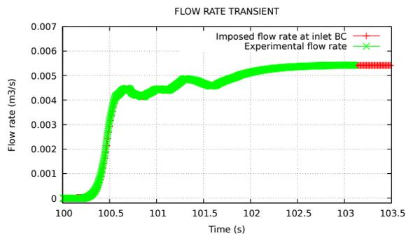
**Figure 10.** Flow rate during fast startup.
