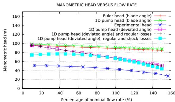
**Figure 6.** Validation of 1D pump ideal and real head prediction.
