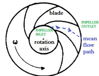
**Figure 2.** Centrifugal rotodynamic pump  $R-\theta$  plane scheme.
