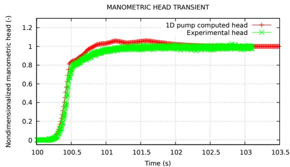
**Figure 12.** Head during fast startup.
