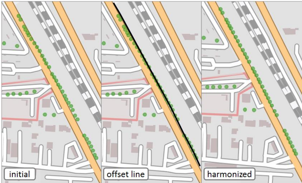
Figure 3: Inaccurate trees overlap a road – harmonization aligns them on a road offset.
