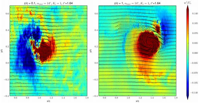
Fig. 4. Velocity field (u'/U<sub>r</sub>,v'/U<sub>r</sub>) with spanwise velocity w'/ U<sub>r</sub> contour, for z/c = 0.1 (left) and z/c = 1 (right).
