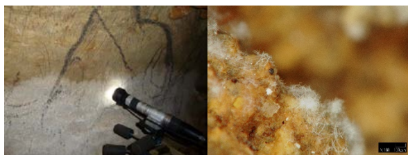
Figure 1. Left: optical microscope at Rouffignac cave lighting a moonmilk layer. Right: calcite needles seen at magnification 160 (scale bar shows 100 microns) at Combarelles cave
