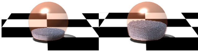
Fig. 9 Left : Simulation of a water balloon upon its impact with the ground using weakly compressible SPH, which suffers from fluid loss. Right : The same scene simulated using our method, which preserves the fluid volume during the simulation. The PBD-stiffness value of the elastic balloon in both simulations is set to 0.80 and stiffness value of WCSPH is 6.0 \times 10^3 .
