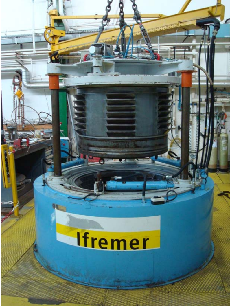
Figure 5. 1000 bar hyperbaric pressure testing chamber.
