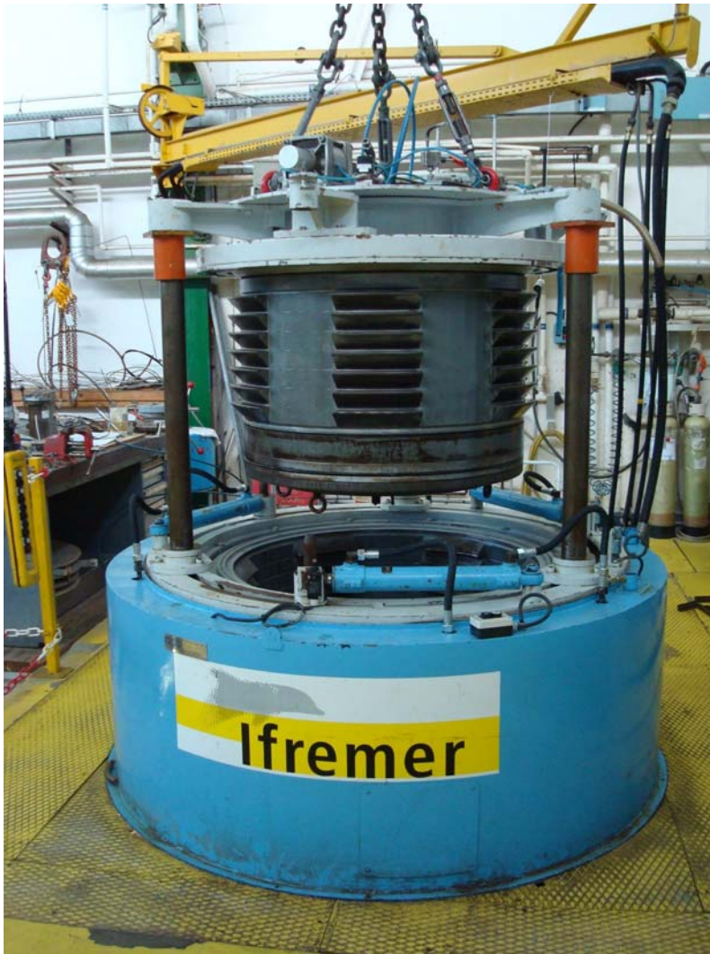
Figure 5. 1000 bar hyperbaric pressure testing chamber.
