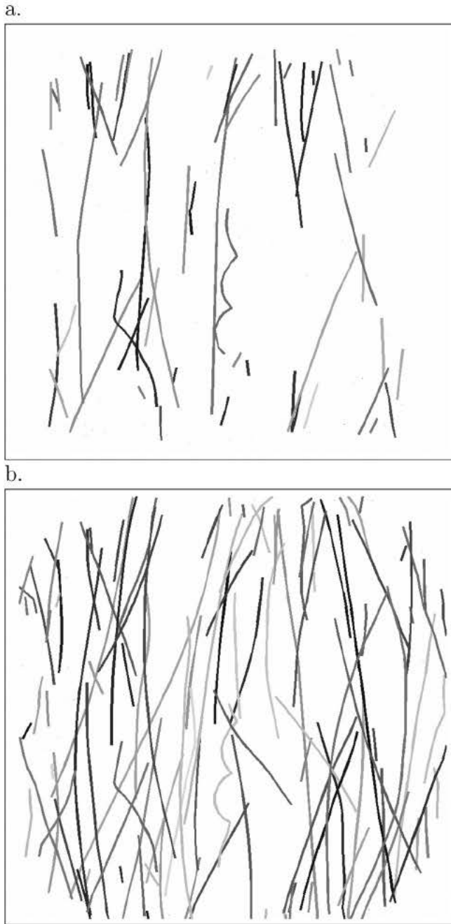
Fig. 13. Trajectories of bubbles for a reduced set of 1500 images with \alpha = 0.5\% . (a) Detection of single bubbles only (algorithm used by Colombet et al., 2011). (b) Detection of single, truncated and overlapping bubbles (present new algorithm).
