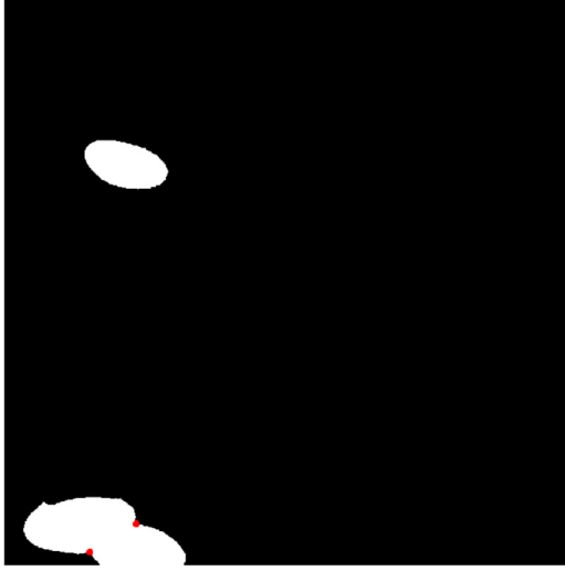
Fig. 8. Binary image of a single bubble and an overlapping bubble. The red points are the inflection points. (For interpretation of the references to color in this figure legend, the reader is referred to the web version of this article.)
