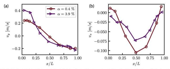
Fig. 9. Vertical liquid velocity  $(v_y)$  and horizontal liquid velocity  $(v_x)$  profiles for different gas volume fractions without the heating. The gas injection is performed at  $x/L \le 0.5$ .
