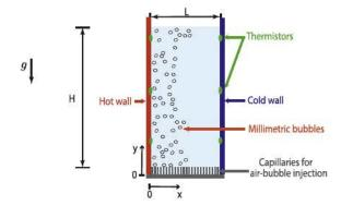
Fig. 1. Rectangular bubbly column heated from one sidewall and cooled from the other (H=500 mm, L=230 mm). Bubbles are injected either close to the hot wall or close to the cold wall, through 90 capillaries (out of 180 in total) placed at the bottom of the setup (inner diameter 0.21 mm).
