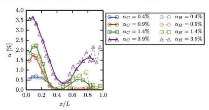
Fig. 3. Gas volume fraction profiles at the mid-height for injection close to the hot wall  $\alpha_H$  and injection close to the cold wall  $\alpha_C$  (cold wall profiles are mirrored around x/L 0.5 for the comparison).
