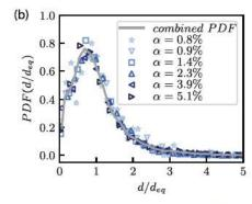
Fig. 4. (a) Mean bubble diameter  $d_{eq}$  for different gas volume fractions  $\alpha$ , the error-bar presents the standard error of the mean bubble diameter. (b) Probability density function (PDF) of the normalised bubble diameter. The symbols present the PDF for each gas volume fraction, while the line presents a PDF calculated using data points for all studied gas volume fractions.
