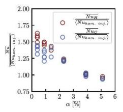
Fig. 7. The ratio of Nusselt for the inhomogeneous bubble injection and Nusselt for homogeneous injection as a function of the gas volume fraction.  $\langle \overline{Nu_{\text{hom inj}}} \rangle$  means averaging over  $Ra_H$  for constant  $\alpha$ .
