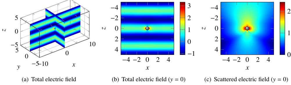
Figure 6: Cross sections of  $x$ -component of the electric field associated to Test 1 with  $\lambda = 5$  and  $\delta = 0.5$ .
