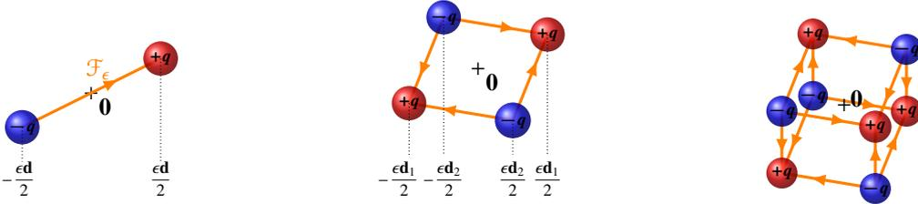
Figure 2: Dipolar, quadrupolar and octupolar configurations
