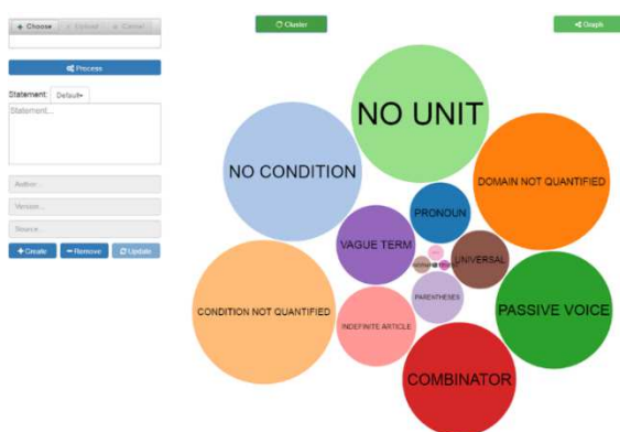
Fig. 3. Clusters of requirements containing quality defects
