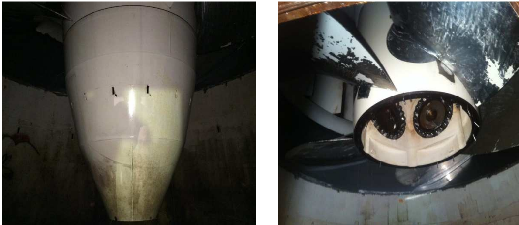
Figure 4: Picture of the cone of the propeller seen from the draft tube, before (left) and after (right) loss.
