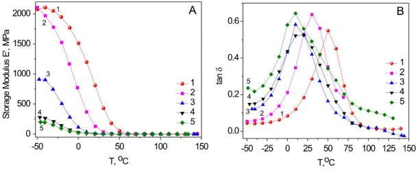
**Figure 6.** Storage modulus (*E'*) (**A**) *vs.* temperature and DMA tan  $\delta$  plots (**B**) of biobased crosslinked latex free films from 100% CBM – 1, 75% CBM and 25% HOSBM – 2, 50% CBM and 50 % HOSBM - 3, 25% CBM and 75% HOSBM – 4, 10 % CBM and 90 % HOSBM – 5.
