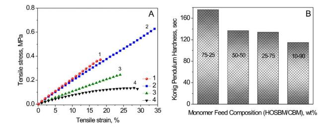
**Figure 7.** Stress-strain plots of biobased latex films from 100% CBM – 1, 50% CBM and 50 % HOSBM - 2, 25% CBM and 75% HOSBM – 3, 10 % CBM and 90 % HOSBM – 4 (**A**). Effect of HOSBM-CBM copolymer composition on pendulum hardness of biobased latex coatings (**B**).
