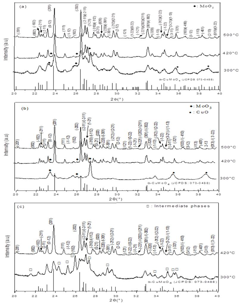
**Figure 3:** XRD patterns of precursors treated at different temperatures: (a)  $P_{Gly}$  treated at 300, 420 and 500°C, (b)  $P_{PAA}$  treated at 300, 420 and 500°C, and (c)  $P_{CAS1}$  treated at 300 and 420°C.
