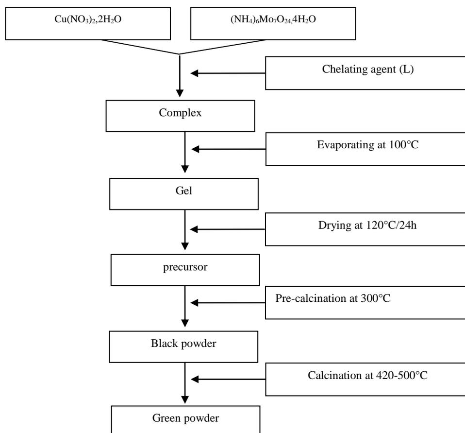
**Figure1:** Flowchart of the synthesis of  $\text{CuMoO}_4$  powder
