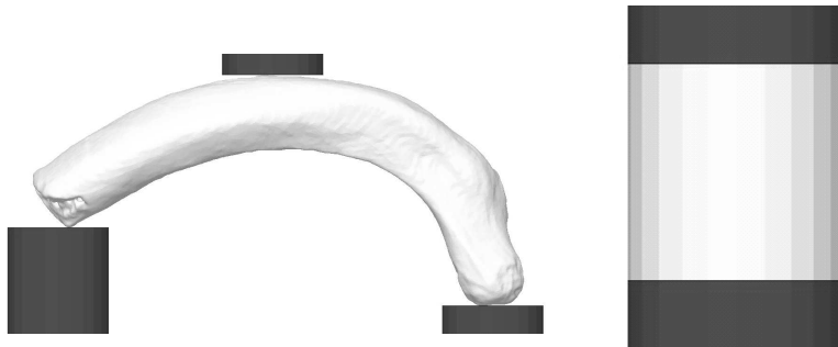
Figure 14: Influence of contact surface. Left: bending rib model. Right: pure compression model (SHPB test).
