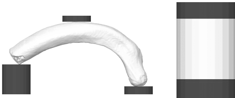
Figure 14: Influence of contact surface. Left: bending rib model. Right: pure compression model (SHPB test).
