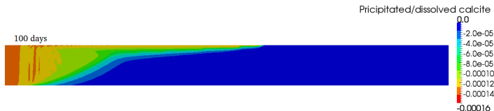
Figure : Precipitated/dissolved calcite volume fraction after 100 days of \text{CO}_2 injection.
