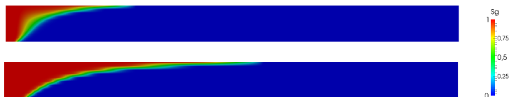
Figure : Saturation S_g after 100 days (top) and 1 year (bas) \text{CO}_2 injection.
