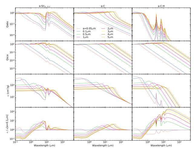
**Fig. 3.** Influence of grain size for compact spherical a-Sil<sub>Fe,FeS</sub> (*left panels*), a-C (*middle panels*), and a-C:H (*right panels*) grains with radius a = 0.05, 0.1, 0.5, 1, 2, 3, 4, and 5  $\mu$ m plotted in pink, blue, green, fuchsia, red, yellow, brown, and orange, respectively. *Top bottom panels*:  $Q_{abs}(a, \lambda), Q_{sca}(a, \lambda), \kappa(a, \lambda)$ , and the ratio of the latter to  $\kappa(a = 0.1 \, \mu m, \lambda)$ .
