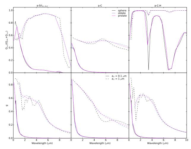
**Fig. 15.** Influence of shape for spherical (black), oblate (blue), and prolate (magenta) a-Sil<sub>Fe,FeS</sub> (*left panels*), a-C (*middle panels*), and a-C:H (*right panels*) grains with radius  $a_V = 0.1$  and  $1 \mu m$ , solid and dashed lines, respectively. *Top panels*:  $Q_{sca}/(Q_{abs} + Q_{sca})$ . *Bottom panels*:  $g = \langle \cos \theta \rangle$ . The asymmetry factor curves appear smoother because the calculations were made for lesser wavelength points.
