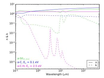
**Fig. 1.** Optical constants of silicates (green), a-C with  $E_g = 0.1 \text{ eV}$  (blue), and a-C:H with  $E_g = 2.5 \text{ eV}$  (fuchsia). The real, *n*, and complex, *k*, parts of the complex refractive index are showed by the solid and dashed lines, respectively.
