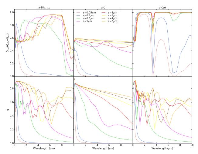
**Fig. 13.** Influence of size for compact spherical a-Sil<sub>Fe,FeS</sub> (*left panels*), a-C (*middle panels*), and a-C:H (*right panels*) grains with radius a = 0.05, 0.1, 0.5, 1, 2, 3, 4, and 5  $\mu$ m plotted in pink, blue, green, fuchsia, red, yellow, brown, and orange, respectively. *Top panels*: albedo  $Q_{sca}/(Q_{abs} + Q_{sca})$ . *Bottom panels*: asymmetry factor of the phase function  $g = \langle \cos \theta \rangle$ .
