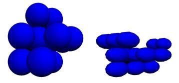
**Fig. 2.** Two examples of aggregate shapes (arbitrary scales). *Left panel*: aggregate made of N = 12 compact spherical monomers with  $a_0 = 0.1 \,\mu$ m. *Right panel*: aggregate made of N = 16 compact prolate monomers with  $a_0 = 0.05 \,\mu$ m and aspect ratios of 2.
