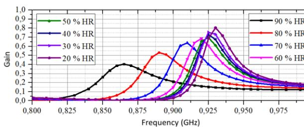
Fig. 5 Antenna gain as a function of humidity
