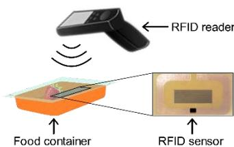
Fig. 1 RFID-sensor concept
