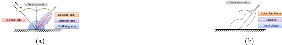
Figure 10: Decomposition of BRDF (a) Phong model-like BRDF decomposition (b) BRDF decomposition following surface state
