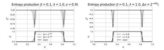
Fig. 3. Local in space numerical entropy production of the advection equation with initial condition  $(I_B)$  for varying space steps  $\Delta x$  at left and for varying relation parameters s at right. The numerical and exact solutions at t=0.1 are shown bellow and the corresponding entropy productions above.
