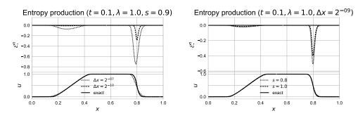
Fig. 5. Local in space numerical entropy production of the Burgers equation with initial condition  $(I_A)$  for varying space steps  $\Delta x$  at left and for varying relation parameters s at right. The numerical and exact solutions at t = 0.1 are shown bellow and the corresponding entropy productions above.
