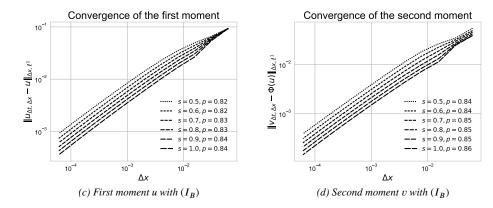
Fig. 4. Error in norm  $\ell^1$  of the numerical solution of the Burgers equation (33) according to the space steps  $\Delta x$  for several relaxation parameter values  $s \in \{0.5, 0.6, 0.7, 0.8, 0.9, 1.0\}$ . p is the convergence rate.
