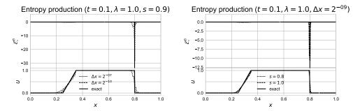
Fig. 6. Local in space numerical entropy production of the Burgers equation with initial condition  $(I_B)$  for varying space steps  $\Delta x$  at left and for varying relation parameters s at right. The numerical and exact solutions at t=0.1 are shown bellow and the corresponding entropy productions above.
