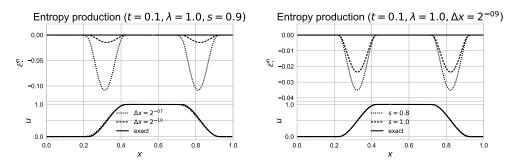
Fig. 2. Local in space numerical entropy production of the advection equation with initial condition  $(I_A)$  for varying space steps  $\Delta x$  at left and for varying relation parameters s at right. The numerical and exact solutions at t = 0.1 are shown bellow and the corresponding entropy productions above.
