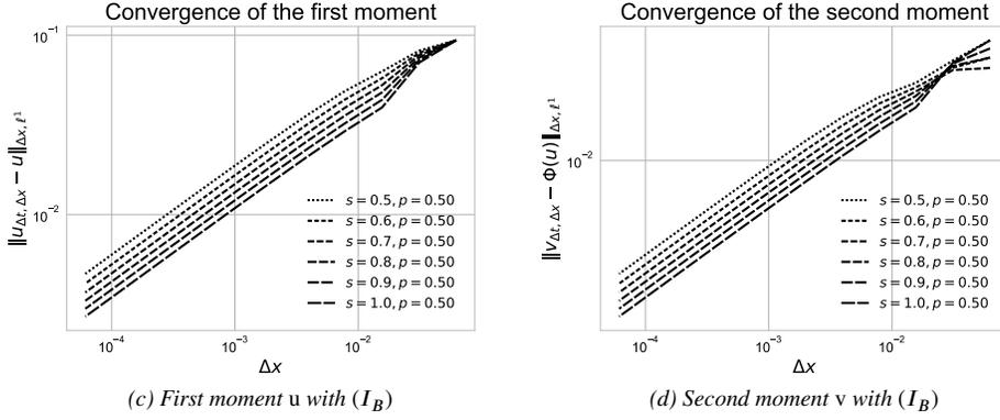
Fig. 1. Error in norm  $\ell^1$  of the numerical solution of the advection equation (32) according to the space steps  $\Delta x$  for several relaxation parameter values  $s \in \{0.5, 0.6, 0.7, 0.8, 0.9, 1.0\}$ .  $p$  is the convergence rate.
