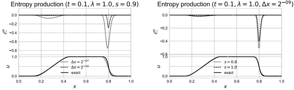
Fig. 5. Local in space numerical entropy production of the Burgers equation with initial condition  $(I_A)$  for varying space steps  $\Delta x$  at left and for varying relation parameters  $s$  at right. The numerical and exact solutions at  $t = 0.1$  are shown below and the corresponding entropy productions above.
