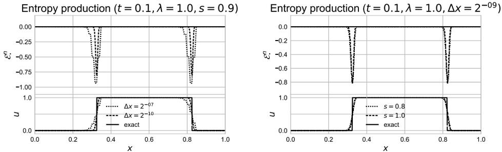
Fig. 3. Local in space numerical entropy production of the advection equation with initial condition  $(I_B)$  for varying space steps  $\Delta x$  at left and for varying relation parameters  $s$  at right. The numerical and exact solutions at  $t = 0.1$  are shown below and the corresponding entropy productions above.
