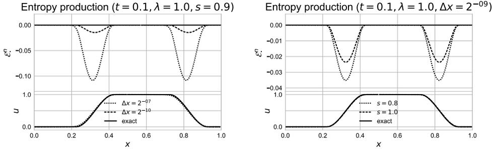
Fig. 2. Local in space numerical entropy production of the advection equation with initial condition  $(I_A)$  for varying space steps  $\Delta x$  at left and for varying relation parameters  $s$  at right. The numerical and exact solutions at  $t = 0.1$  are shown below and the corresponding entropy productions above.
