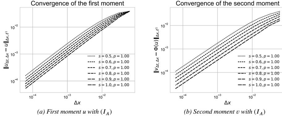
Fig. 4. Error in norm  $\ell^1$  of the numerical solution of the Burgers equation (33) according to the space steps  $\Delta x$  for several relaxation parameter values  $s \in \{0.5, 0.6, 0.7, 0.8, 0.9, 1.0\}$ .  $p$  is the convergence rate.
