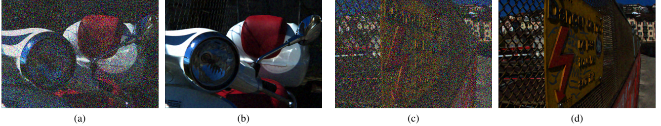
Fig. 9: 4D tensor driven diffusion is able to denoise highly damaged light fields. Center views for Vespa and DangerDeMort from the EPFL dataset [33]. (a,c) With Additive Gaussian noise ( \sigma = \frac{100}{255} , overall PSNR 8.13 dB); (b,d) After denoising giving a PSNR of 29.31 dB (b) and 28.50 dB (d).
