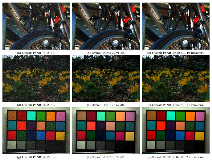
Fig. 10: Denoising of the *Bikes*, *Flowers* and *Color Chart 1* light fields [33]. Center views. (a,d,g) Gaussian noise of  $\sigma = \frac{50}{255}$ . (b,e,h) Result obtained using LFBM5D with parameterization provided by the authors [2]. (c,f,i) Using our method. An extended quantitative comparison with other methods can be found in Table I.
