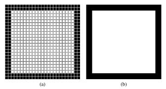
Fig. 1: Tesseract as a 4D light field toy example: (a) Set of  $25 \times 25$  light field views; (b) Subaperture image of 25x25 pixels image containing a square at the center of 21x21 pixels for the central views (fully black image at the periphery of the light field).
