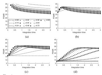
Fig. 4: Denoising behaviour for different noise levels applied to the *Bikes* light field. Each curve represents the PSNR evolution along the diffusion iterations, for different values of the parameter  $\rho_r$ , in the cases of (a) No noise; (b) additive Gaussian noise with  $\sigma = \frac{10}{255}$ ; (c)  $\sigma = \frac{40}{255}$ ; and (d)  $\sigma = \frac{100}{255}$ . The parameter  $\alpha$  controlling the anisotropy is set to 2.
