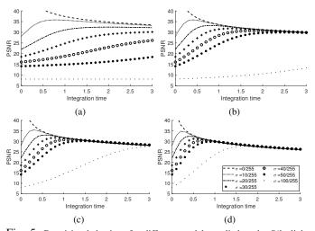
Fig. 5: Denoising behaviour for different models applied to the *Bike* light field of the *EPFL* dataset [33]. Each curve represents the PSNR evolution along the diffusion iterations for different noise standard deviations  $\sigma_G$ , using a model parameterized by (a)  $\rho_r = 0.16$ ; (b)  $\rho_r = 0.32$ ; (c)  $\rho_r = 0.48$ ; (d) and  $\rho_r = 0.80$ . The parameter  $\alpha$  controlling the anisotropy is set to 2.
