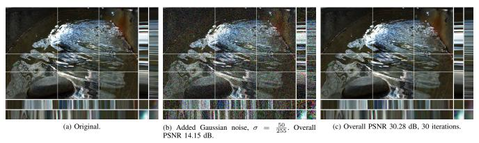
Fig. 18: Denoising results with the *Fountain Pool* light field [33], containing non-Lambertian surfaces. The denoising model is parameterized by  $\rho_4 = 0.4$ ,  $\rho_3 = \frac{1}{2}\rho_4$ ,  $\rho_2 = \frac{1}{4}\rho_3$ , and  $\rho_1 = \frac{1}{8}\rho_2$ . Epipolar plane images are stretched in the angular direction by a factor 4 for sake of clarity. Best viewed zoomed.
