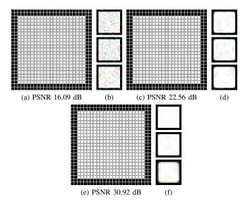
Fig. 7: Denoising of the Tesseract toy example. (a,b) Gaussian noise added to tesseract example (standard deviation  $\sigma = \frac{40}{255}$ ). (c,d) After 20 iterations, using the 2D denoising method proposed in [8]. (e,f) After 30 iterations using the proposed 4D denoising model. PSNR computed over all images.
