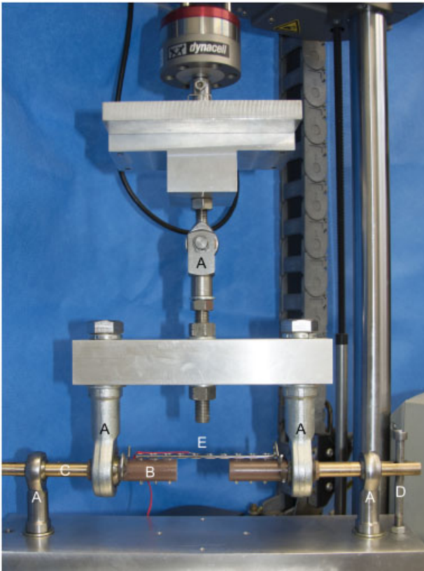
Fig. 2 Photograph of the mechanical setup. (A) Spherical joints; (B) bone substitute; (C) bronze rod; (D) partial thread screw avoiding axial rotation of the bone plate constructs during the tests; (E) strain gauge.
