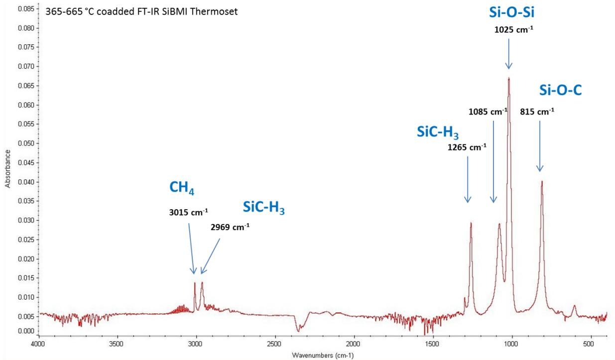
Figure 7 : FTIR spectrum of SiBMI thermoset during TGA between 365 and 665 °C (coadded spectrum)
