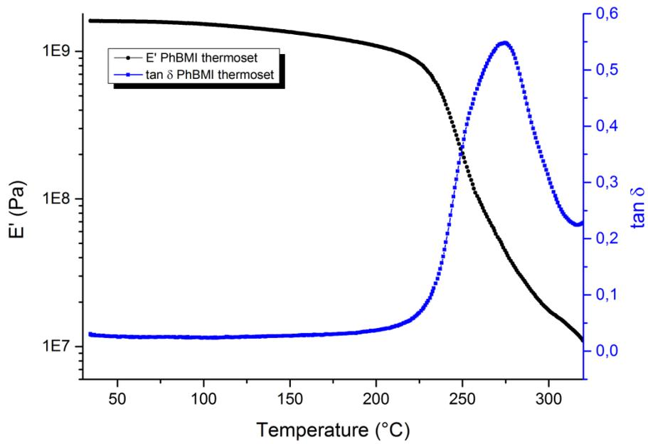
Figure 4:  $E'$  (dots) and  $\tan \delta$  (squares) of DMA curves for PhBMI thermoset.
