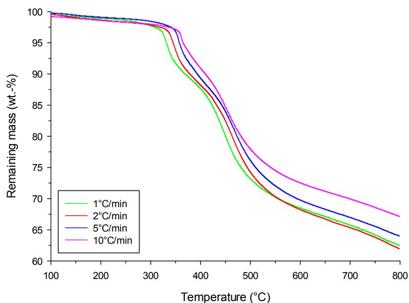
Figure 12 - TG curves of PhBMI thermoset as a function of heating rate (N<sub>2</sub> flow)
