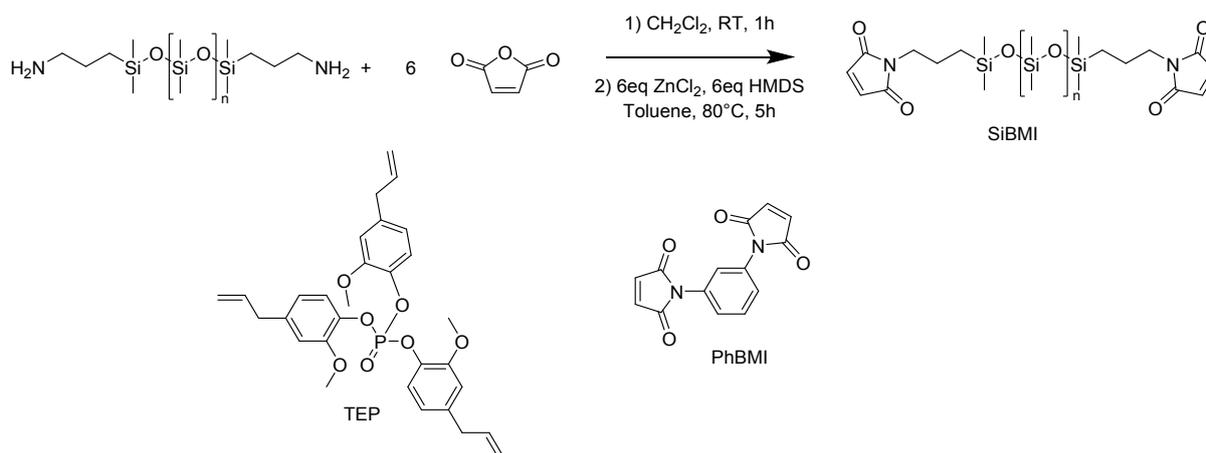
Scheme 1 : Synthesis of SiBMI and chemical structures of TEP and PhBMI.
