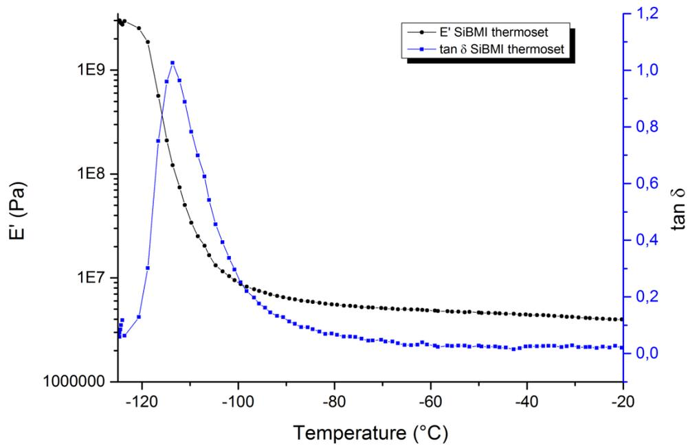
Figure 5:  $E'$  (dots) and  $\tan \delta$  (squares) of DMA curves for SiBMI thermoset.
