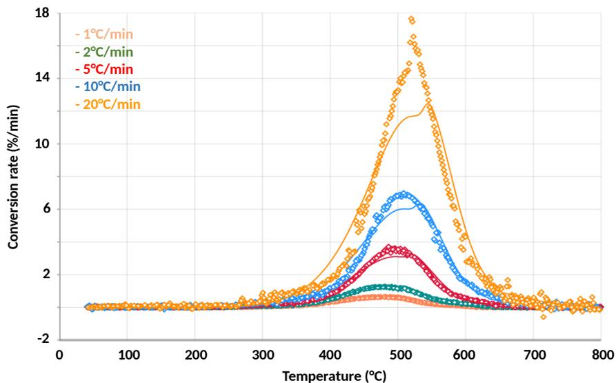
Figure 11 - Experimental and simulated DTG curves of SiBMI thermoset
