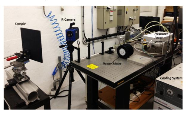
Figure 3: Experimental setup representing the front face flash method.
