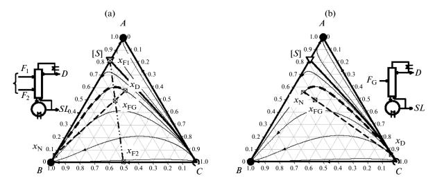
Fig. 8. Indirect separation (a) and direct (b) azeotropic continuous distillation.
