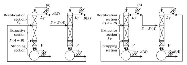
Fig. 5. Flowsheet of typical extractive distillation with (a) heavy entrainer, (b) light entrainer.
