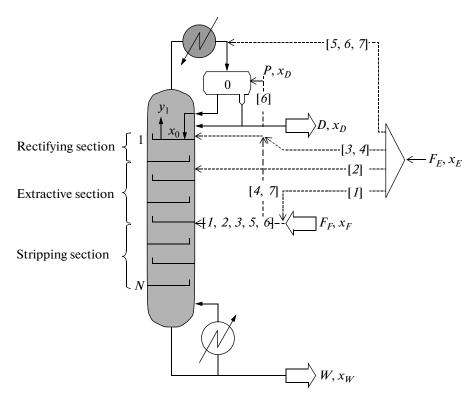
Fig. 6. Configurations for the heterogeneous extractive distillation column considering all possibilities for both the entrainer recycle and the main azeotropic feed.
