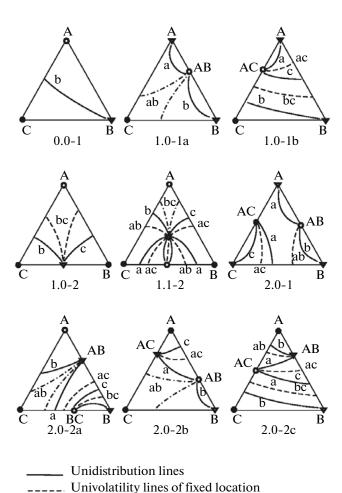
**Fig. 2.** Unidistribution and univolatility line diagrams for the most probable classes of ternary mixtures according to
