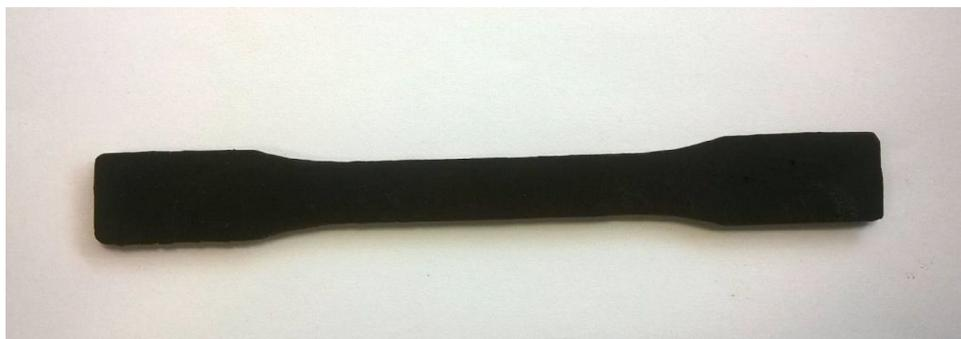
**Fig. 2.** PU film sample for stress-strain testing
