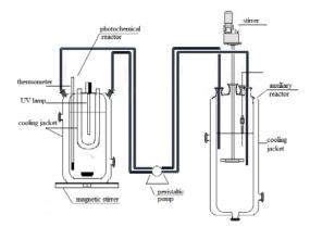
Fig. 1. Experimental set-up for photolysis,  $UV/H_2O_2$  and photo-Fenton oxidation.
