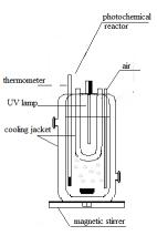
Fig. 2. Experimental set-up for heterogeneous photocatalytic degradation.
