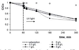
Fig. 3. Photocatalytic degradation of paracetamol at different  ${\rm TiO}_2$  concentrations.
