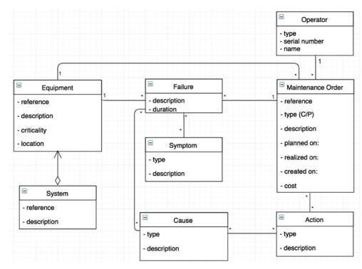
Fig. 4. Basic model of a maintenance order (Grabot, 2017).
