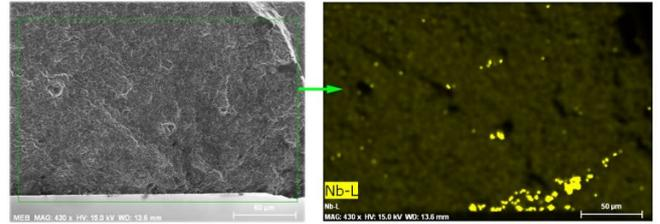
Fig. 9 Example of niobium mapping on crack initiation site obtained using Energy Dispersive X-ray Spectroscopy (EDS). A cluster of niobium carbides is clearly visible
