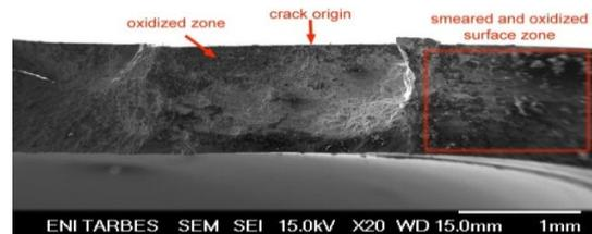
Fig. 10 SEM observation of a rupture facies in the case of a tension-compression test ( $T=0.48$ ). Smeared surface structures and oxidized zones (dark zones) are observed. Crack initiates from subsurface carbides and spread out elliptically through the thickness of the specimen
