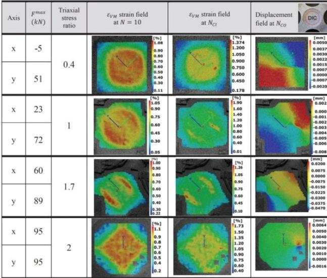
Fig. 5 Test results. Plots of the equivalent von Mises strain field at the beginning of each test ( $N=10$ ), at crack initiation ( $N=N_{ci}$ ) and plot of the displacement field at crack opening ( $N=N_{co}$ )
