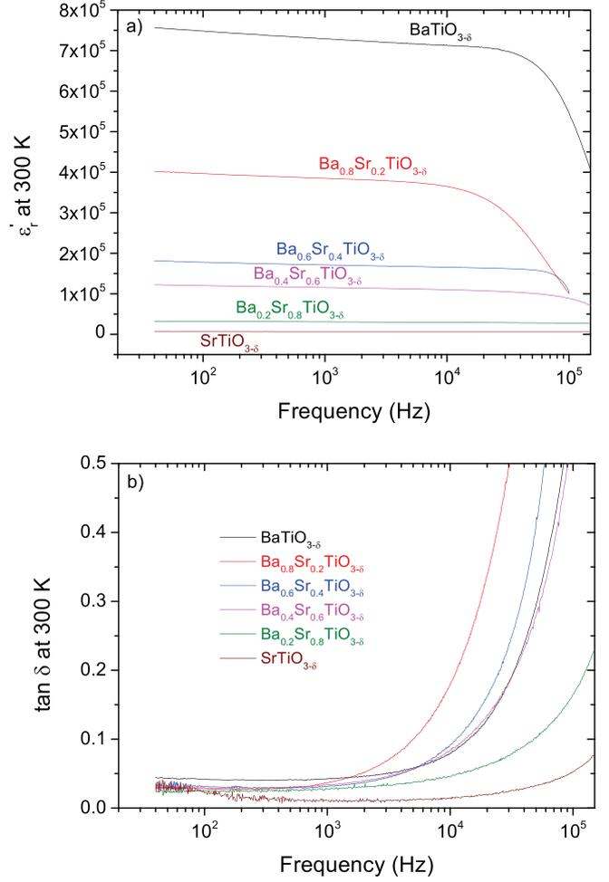
**Fig. 4.** Variation of the real part of relative permittivity (a) and losses (b) as a function of frequency for the  $\text{Ba}_{1-x}\text{Sr}_x\text{TiO}_{3-\delta}$  nanoceramics at 300 K.
