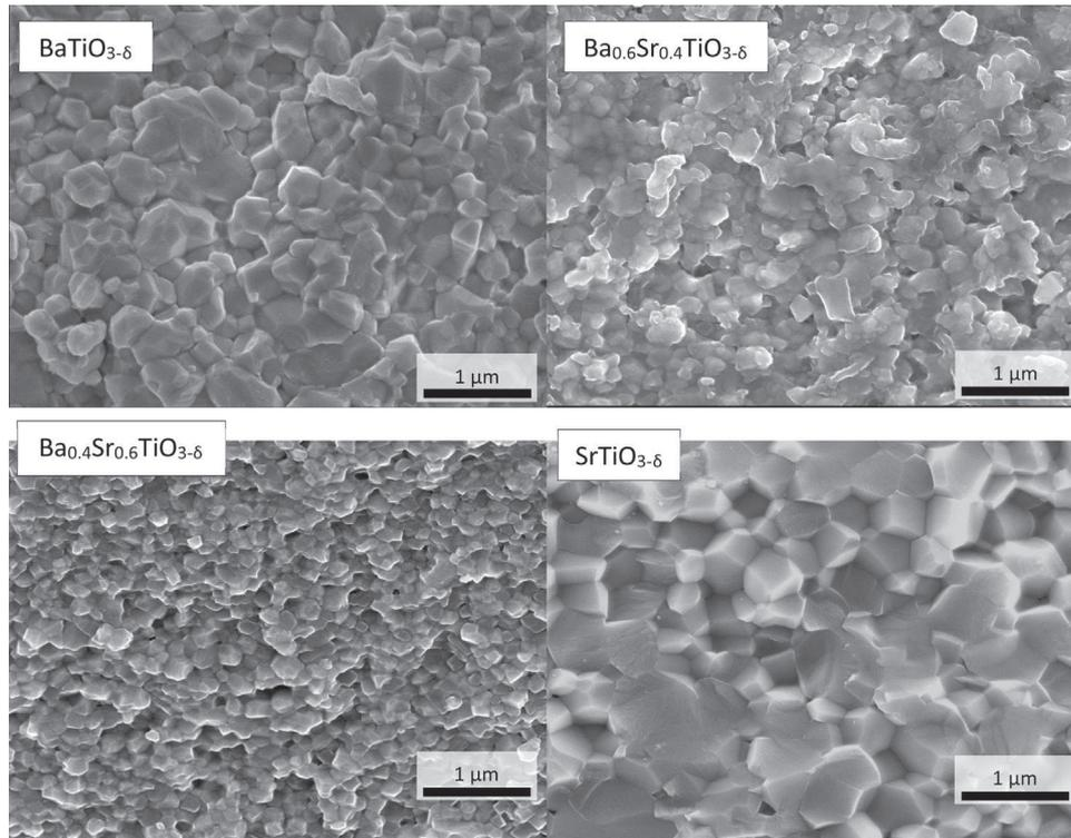
**Fig. 2.** FEG-SEM micrographs of  $Ba_{1-x}Sr_xTiO_{3-\delta}$  fractured dense ceramics.
