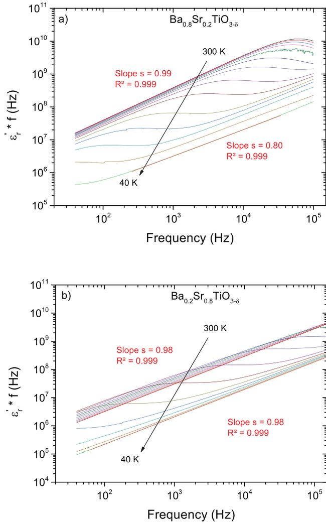
**Fig. 9.**  $\epsilon'' \times f$  vs.  $f$  plot in log-log scales for (a)  $\text{Ba}_{0.8}\text{Sr}_{0.2}\text{TiO}_{3-\delta}$  and (b)  $\text{Ba}_{0.2}\text{Sr}_{0.8}\text{TiO}_{3-\delta}$  dense nanoceramics at different temperatures (40–300 K).
