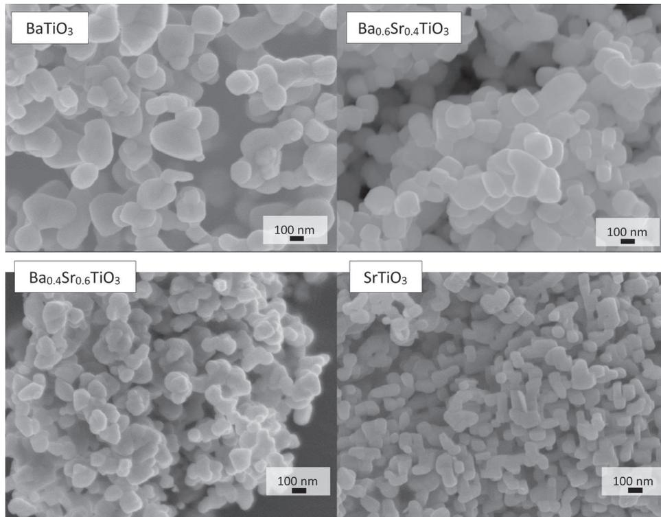
Fig. 1. FEG-SEM micrographs of Ba<sub>1-x</sub>Sr<sub>x</sub>TiO<sub>3</sub> powders.
