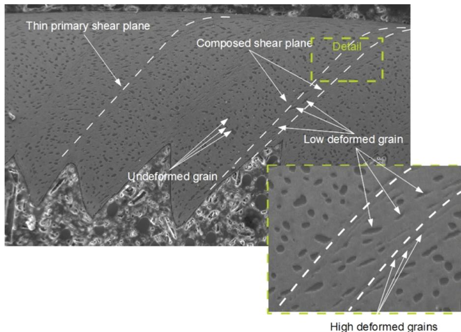
Fig. 1 Chip formation during Ti5553 turning [8]
