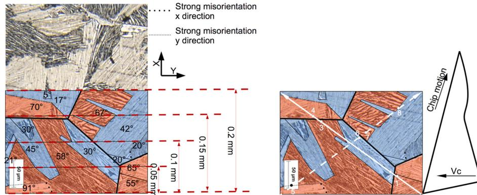
Fig. 12 Effect of feed on chip formation
