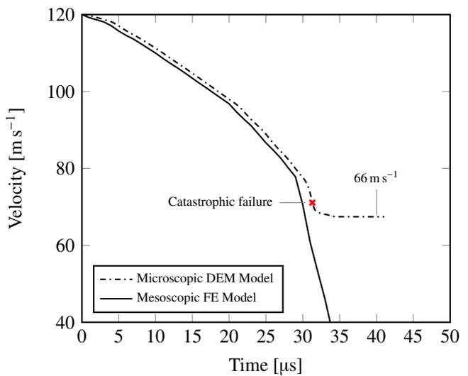
**Figure 6.** Projectile velocity comparison for a transverse impact at  $120 \text{ m s}^{-1}$ .
