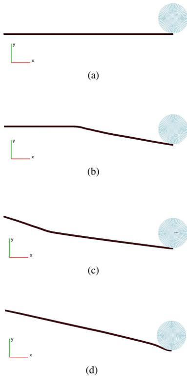
**Figure 4.** Impacted Yarn using FEM
