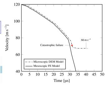
Figure 6. Projectile velocity comparison for a transverse impact at  $120 \text{ m s}^{-1}$ .
