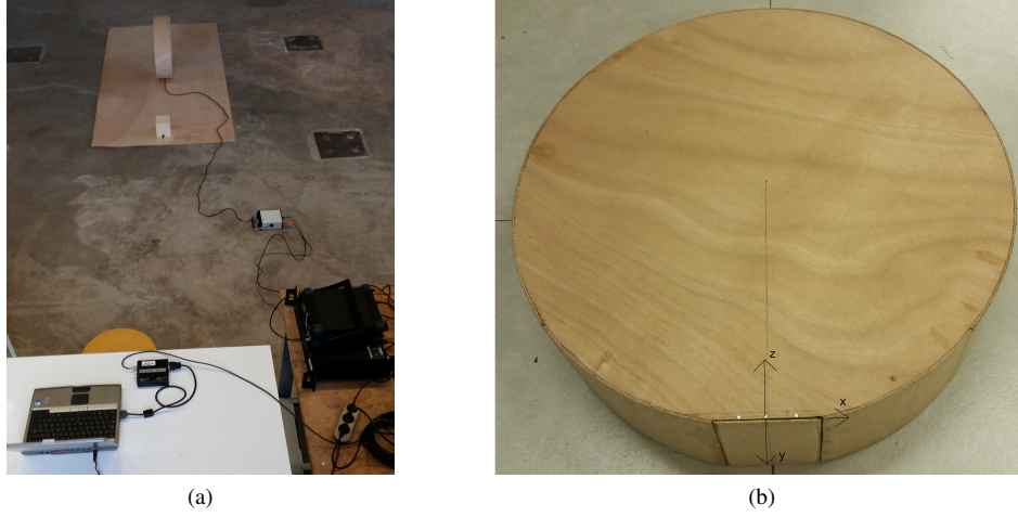
Figure 9: (a) The experimental set-up; (b) flange used in the calculations and experiments
