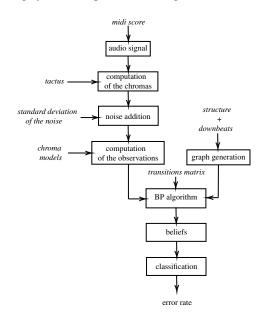
Figure 5. Flowchart of the test system for estimating the robustness to noise
