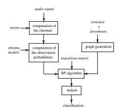
Figure 1. Flowchart of our system. Italic represents the the input of the system, and each box corresponds to a part of the signal processing that is detailed in the corresponding section.
