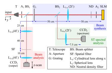
**Figure 2** | Schematic depiction of the optical setup for synthesis and analysis of a ST wave packet. The inset provides a key for the optical components. The various sections of the setup are identified with differently colored backgrounds.
