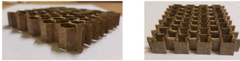
Figure 2. Hexagonal cell honeycomb (left) and re-entrant (auxetic) cell honeycomb (right) resulting from the Kirigami manufacturing.
