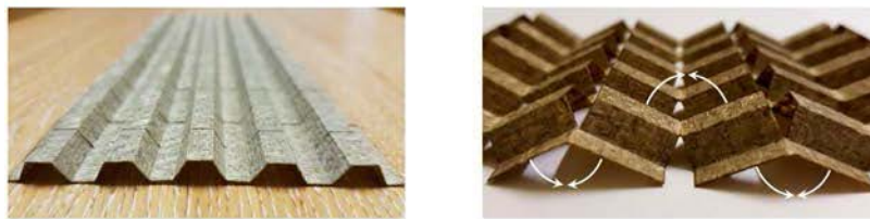
Figure 1. Hexagonal cell honeycomb: corrugated sheet after the thermoforming and laser cutting of the slits (left) and after folding along the slits (right).
