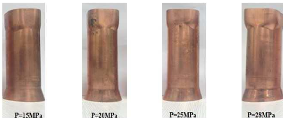
Figure 4: Tube after expansion in a square die with various internal pressures: experimental results.
