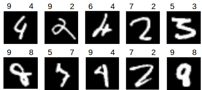
Fig. 7. Examples of wrongly classified digits by an ESN of 1,000 neurons with a joined state output layer. Digits on the top-left side are the digits found by the ESN, and the one on the top-right side are the real digits found in the MNIST database.
