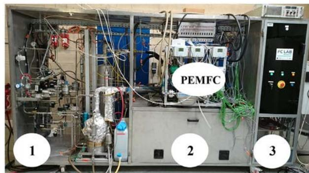
**Fig. 1 – 10 kW test bench.**
