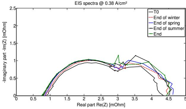
**Fig. 11 – Ageing impact on the EIS measurements.**
