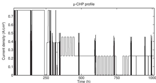
Fig. 4 – 1000 h  $\mu$ -CHP load profile.
