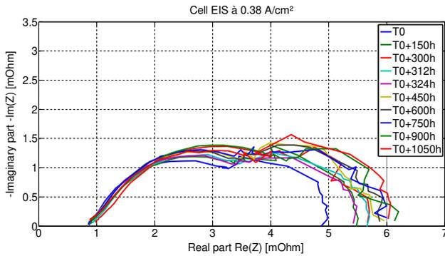
Fig. 7 – Ageing impact on the EIS measurements (1000 h).
