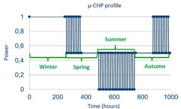
Fig. 3 –  $\mu$ -CHP normalized power profile.
