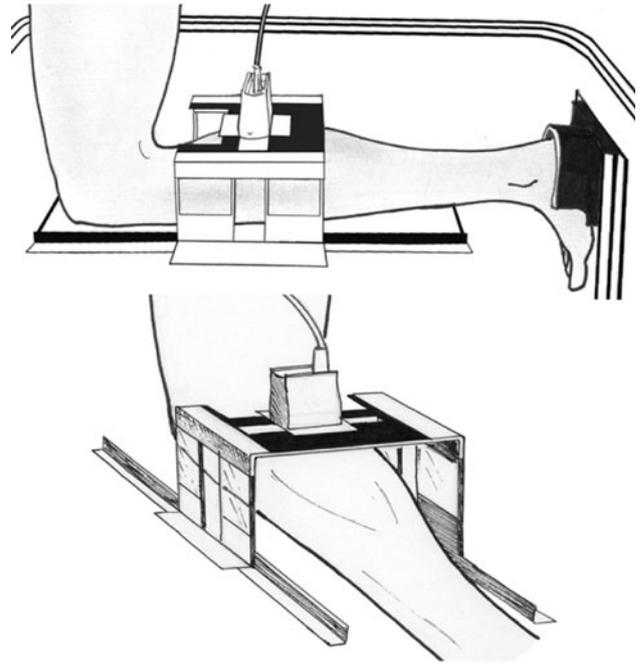
**Fig. 1** Subject position for ultrasound scanning in the water-field container (cut away). The subjects were kneeling and water covered the entire lower leg. The foot was rigidly stabilized at  $90^\circ$  of ankle flexion. Knee angle was maintained at  $90^\circ$  of knee flexion by having the leg supported at the end of the water-field container. Ultrasound images were acquired transversally on each side of the lower leg using a specific probe guide
