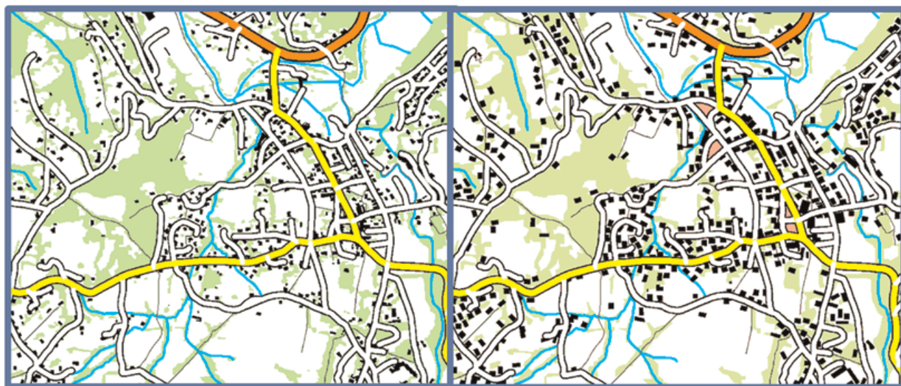
Figure 4. Un-generalized (left) and generalized (right) 1:50k topographic map (429 and 1459 measured values for edge density) Source: IGN
