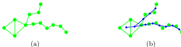
Fig. 6: General illustration of the extraction of a dual mesh in areas of the mesh where primal faces and edges are connected. (a) This primal mesh has been generated from a previous iteration. It generates mixed meshes with edges and faces. (b) The dual mesh in blue is generated mostly by using the standard rules explained earlier. However, in mixed areas, dual vertices in edges have to be connected to dual vertices in primal faces generating a junction.
