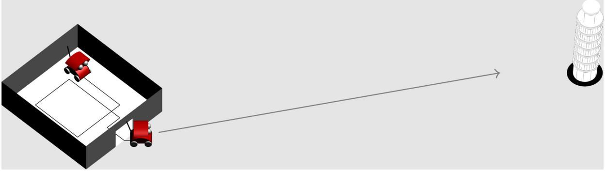
Fig. 3: Numerical experiment. A robot having unknown initial position and orientation explores a room, and builds a map of 8 characteristic *unknown* features. Then, it leaves the building until it observes the bearing of a clearly visible landmark with *known* location (the Pisa tower). This new observation brings information about its position and orientation, and consequently on the general orientation and origin of the map it has built.
