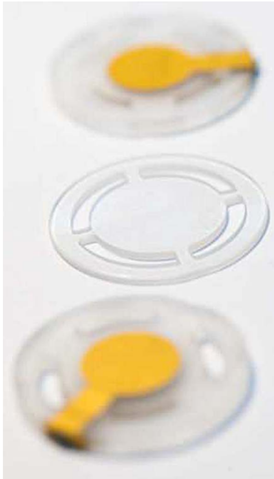
FIG. 1. Quartz crystal resonator with electrode holders (Photo: L. Godard, UFC Besançon, France). The plano-convex BAW cavity located in the center of the structure, in the middle of the photography, is partly isolated from external mechanical disturbances by means of four “bridges” linking the active part to its rim. The two metallized quartz parts at the top and bottom of the photography are optional actuating electrodes which can be placed at a distance of about 1\ \mu\text{m} on both sides of the BAW cavity when the central structure is sandwiched between these electrode holders. Alternatively, the BAW cavity part can be metallized itself to form an optical cavity colocalized with the mechanical one.
